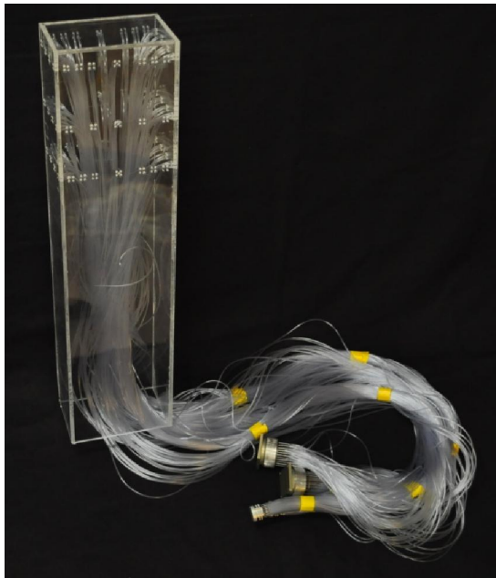
Figure 4. Wind tunnel model of the CAARC standard tall building with pressure taps.
